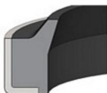
**Raschiatore AM 45 (NBR 90/METAL)**
